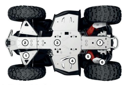
For ultimate durability and strength, all our Aluminum Skid Plates are made with %6" (4.5 mm) thick High Strength 5052 H32 Aluminum.
