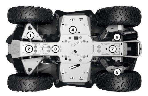
For ultimate durability and strength, all our Aluminum Skid Plates are made with 3/16" (4.5 mm) thick High Strength 5052 H32 Aluminum.
