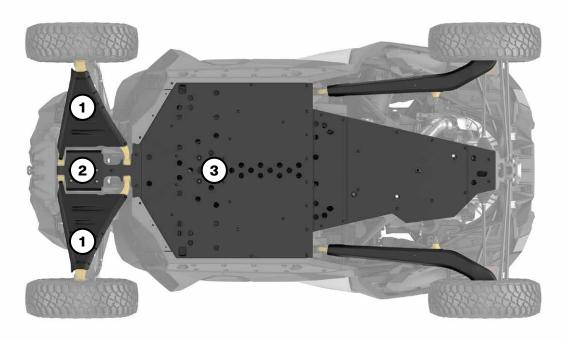
Our plastic plates glide smoothly and silently over obstacles, offering great protection in rough terrain. Made of abrasion-resistant thermoformed %" (10 mm) thick High Molecular Weight Polyethylene (HMWPE).
